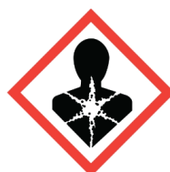
Specific Toxicity Hazards
