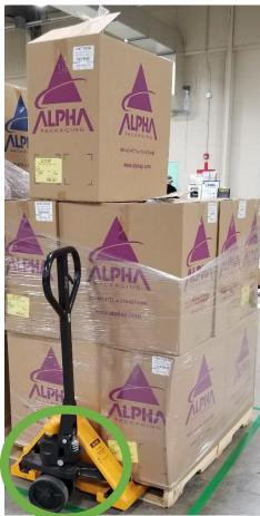
Jacks must always be parked inside of a pallet with its turning wheels fully turned to one side as shown.
